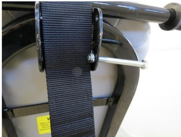
**Step 2:** Put the new shoulder in place; then place the long bent leg of the cam spring into the tiny hole in the buckle (Welded to the chair), and hold it in place with the tip of a 7mm bolt. The long bent leg must be against the outside of the buckle, and the short leg of the cam spring must be facing the inward side of the buckle (Slightly over the webbing).
