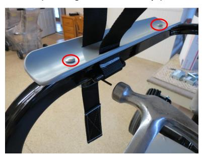
**Step 4:** Put the new arm in place and slide the small loop over the arm clevis. Two carriage bolts go through the arm and "seat" into the arm. Tap an eighth inch roll pin into the arm clevis until flush (This prevents the strap from being removed by detainees).
