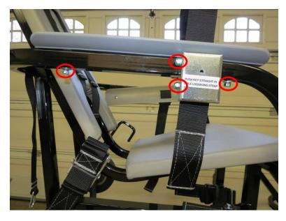
**Step 1:** Remove the four nuts from each side of the chair. Two from the carriage bolts on the underside of the arms, and two from the 7mm bolts holding the chrome buckle cover in place. Then remove the top 7mm bolt and take the chrome buckle cover off.
