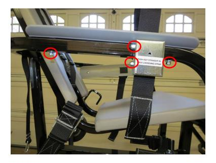
**Step 8:** Place a flat washer, split washer, and nut on the carriage bolts and tighten. Place a nylon lock nut on the 7mm bolts, but do not over tighten.
