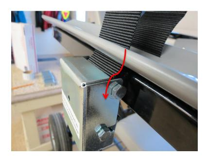
**Step 7:** Push the buckle cover into place (Slotting into the bottom 7mm bolt). Then install the top 7mm bolt through the buckle *behind* the webbing.
