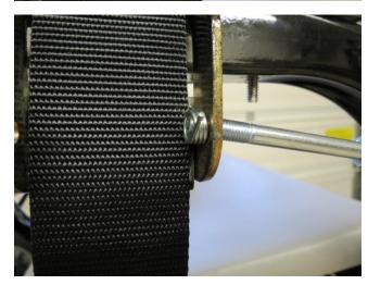
**Step 5:** Place the long bent leg of the cam spring into the tiny hole in the buckle (Welded to the chair), and hold it in place with the tip of a 7mm bolt. The long bent leg must be against the outside of the buckle, and the short leg of the cam spring must be facing the inward side of the buckle (Slightly over the webbing).
