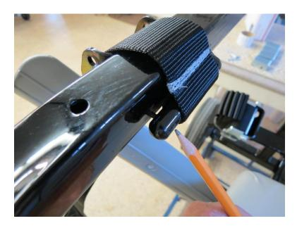
**Step 3:** With an eighth inch punch or nail, hammer the roll pin into the arm of the chair and slide the looped end of the arm strap off the arm clevis.
