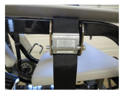
**Step 6:** Push the cam into the buckle making sure to catch the short leg of the cam spring behind the cam; then slide the 7mm bolt all the way through the buckle.
