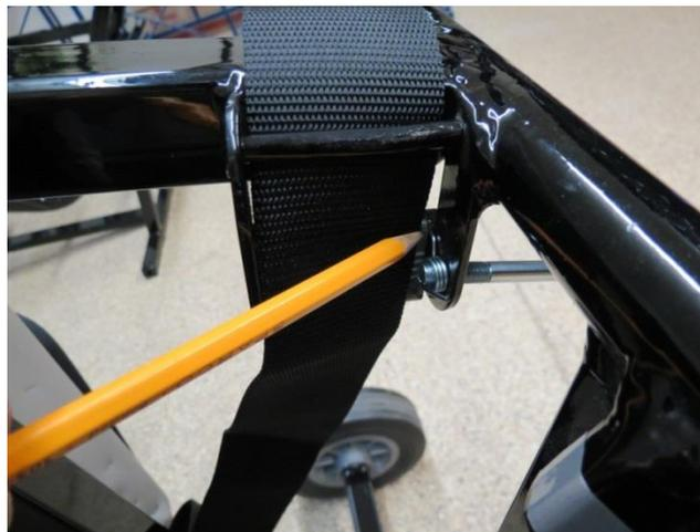
**Step 4:** On the left ankle buckle, place the long bent leg of the cam spring into the tiny hole in the buckle (Welded to the chair), and hold it in place with the tip of a 7mm bolt. The long bent leg must be against the outside of the buckle, and the short leg of the cam spring must be facing the inward side of the buckle (Slightly over the webbing).
