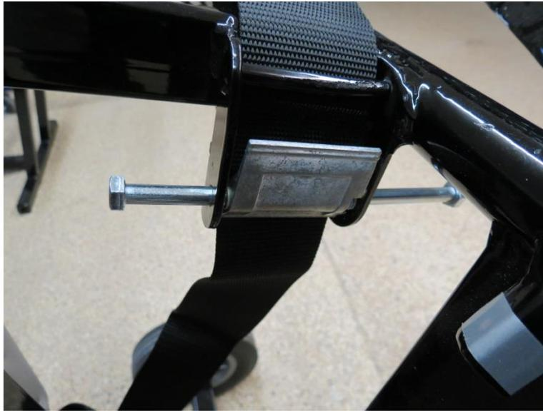
**Step 5:** Push the cam into the buckle making sure to catch the short leg of the cam spring behind the cam; then slide another 7mm bolt through the buckle from the topside. Line up the bolts and tap the top bolt through the buckle quickly so that it pushed the bottom bolt out. Place a nylon lock nut on the 7mm bolt, but do not over tighten.
