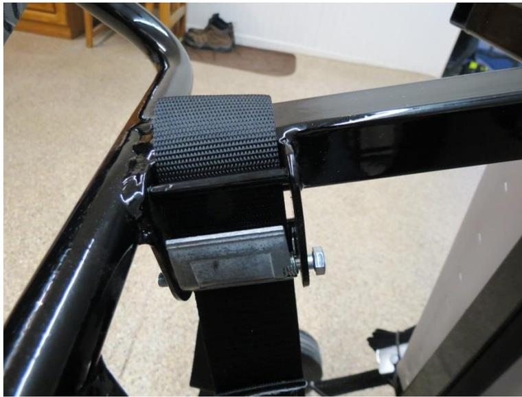
**Step 7:** Push the cam into the buckle making sure to catch the short leg of the cam spring behind the cam; then slide the 7mm bolt all the way through the buckle. Place a nylon lock nut on the 7mm bolt, but do not over tighten.
