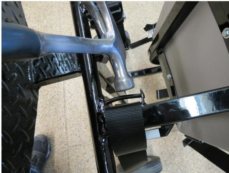
**Step 3:** Pass the small end of the ankle strap up from the bottom through the space you created (The handle end should be pointing to the back or downward). Tap the strap guide back so that it's straight.
