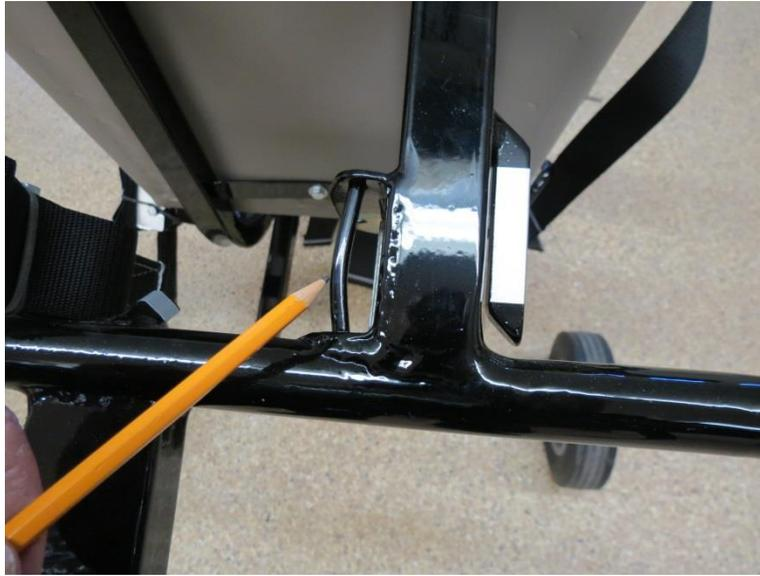
**Step 2:** The strap guide is welded in place at the front of the buckle and needs to be bent slightly inward so the strap can be removed. A claw hammer or small crowbar works well for this.
